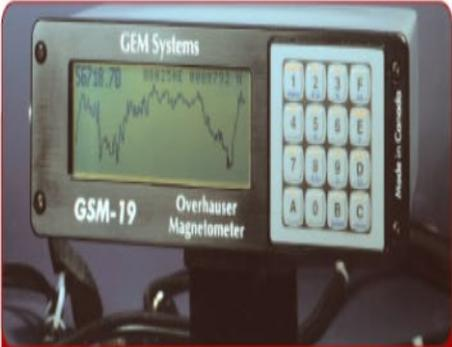
Overhauser (GSM-19W) Walking Magnetometer console. Can also be configured with additional sensor for gradiometer (simultaneous) readings.
