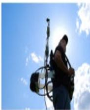
Walking Gradiometer with VLF-EM and GPS
